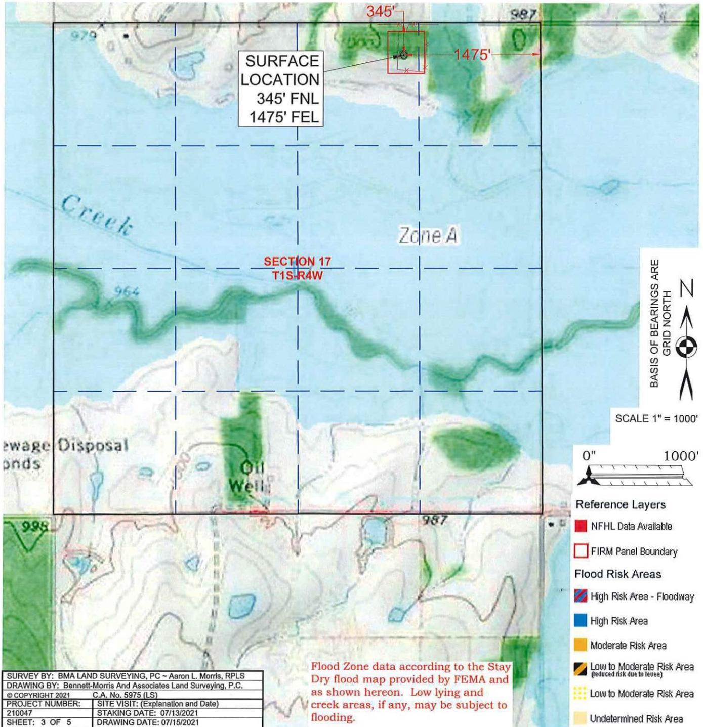
Flood Zone data according to the Stay Dry flood map provided by FEMA and as shown hereon. Low lying and creek areas, if any, may be subject to flooding.
