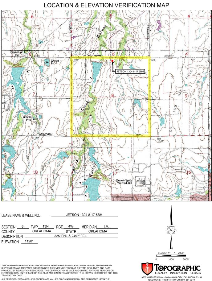
ALL BEARINGS, DISTANCES, AND COORDINATE VALUES CONTAINED HEREON ARE GRID BASED UPON THE OKLAHOMA STATE PLANE COORDINATE SYSTEM, NORTH ZONE OF THE NORTH AMERICAN DATUM 1927, U.S. SURVEY FEET AND THE NATIONAL GEODETIC VERTICAL DATUM OF 1929.
