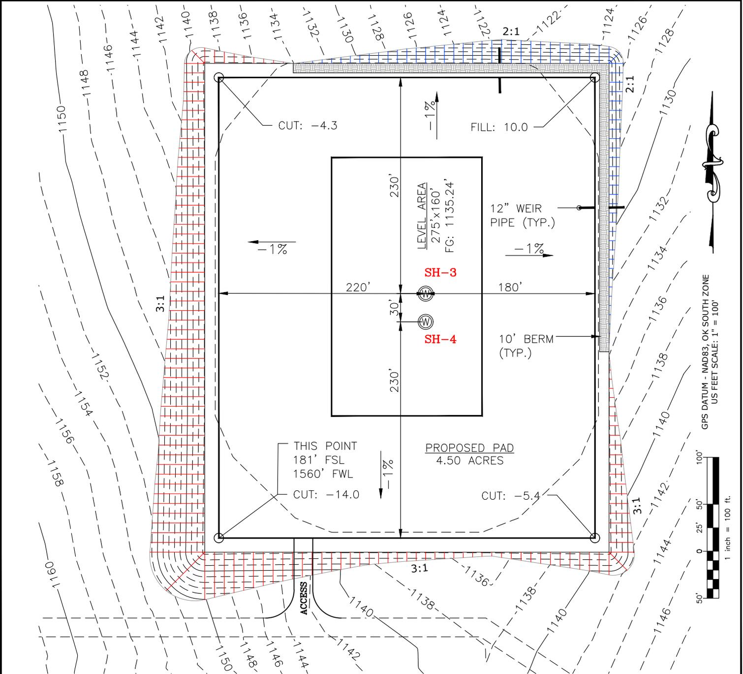
CUT VOLUME 22133.66 CU. YD. | 6" OF STRIPPED TOP SOIL: 4,948.48 CU. YD.
